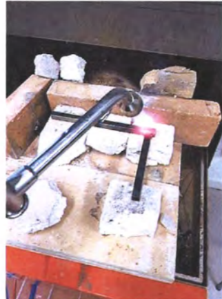
Brazing the bar to the leg, which failed as the brass kept reaching melting point before the bar secured to the leg
