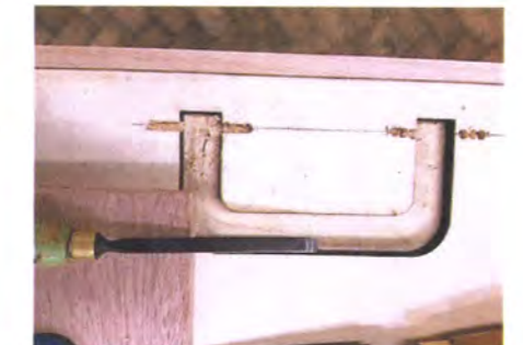
Chiselling out the space where the mechanism will be fitted
