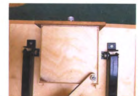
Securing the stoppers to the base of the legs to keep the legs in place when the stool is in use
