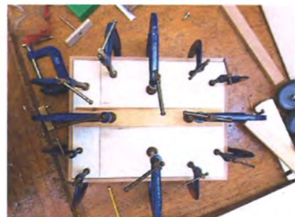
Gluing the formica laminate onto the seat
