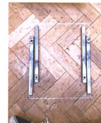
A sketch on the floor to work out where to braze a bar to the legs
