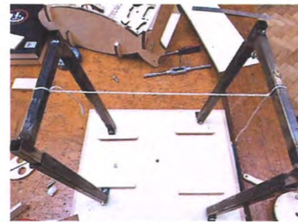
Testing a string method for preventing the legs from moving further outwards while in use
