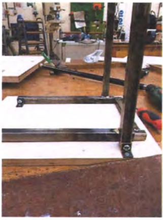
Testing to see that the legs move smoothly
