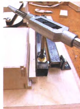
Removing the brass from inside the brazed nut
