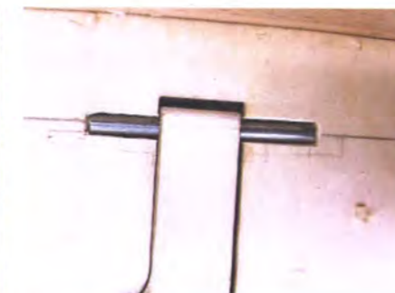
Securing the handles to the seat with glue
