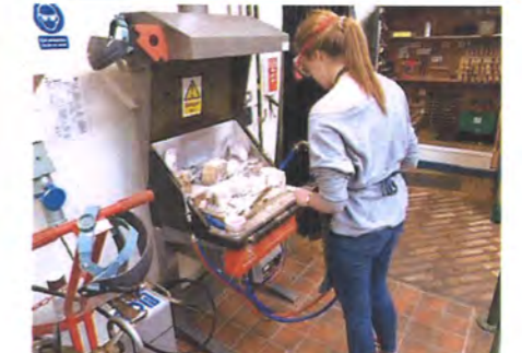
Brazing a nut onto the leg for the height adjustment mechanism
