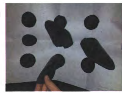
Although the holes were evenly spaced out, they were mostly clustered in the middle of the paper meaning that the centre was weakened when the tools were put in place. Also, depending on the tools stored, they could clash with each other making this layout unsuitable. ②
