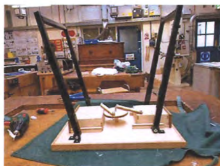
Gluing the formica laminate onto the seat
