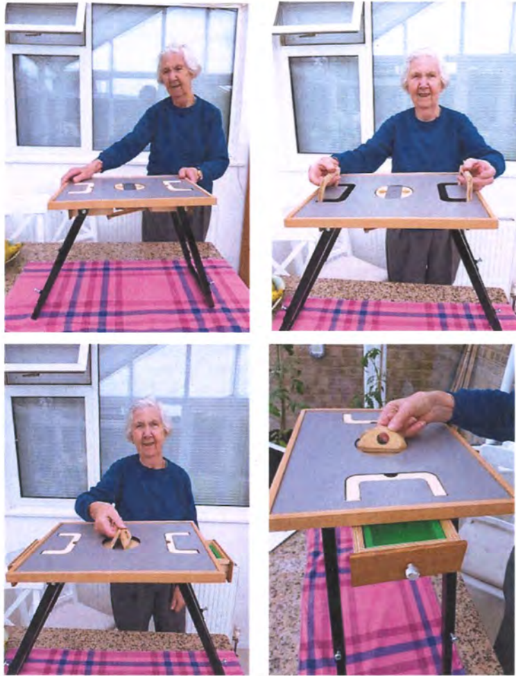
My client testing the handles on the prototype, and turning out the drawers
