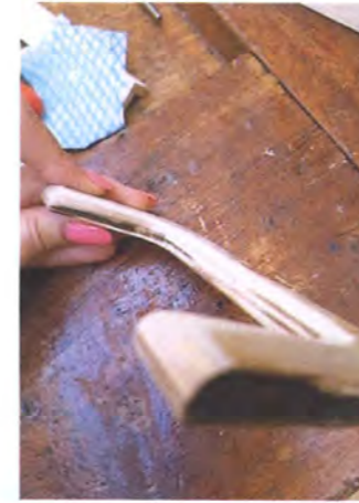
Sanding down the harsh edges of the handles
