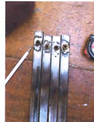
After brazing nuts onto all the legs
