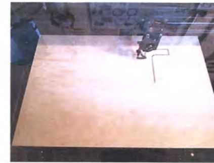
Laser cutting the seat
